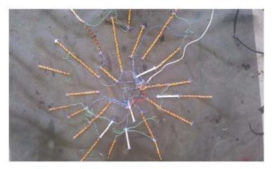
6. Once everything is tested and done, connect a main power lead to each of the 3 channels (just leave it dangling for now) and solder over all connections. I also found liquid electrical tape to be a god send here. Do the same for the middle and outer rings.
